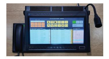
The digital radio dispatch center (D-RDC) is designed to be fully compatible with the existing analog dispatch center by supporting the all currently used services with the possibility to easily add new ones. This enables easy replacement of existing analog dispatch center with the new D-RDC systems, without any modifications done on modulation lines, fixed railway radio stations and mobile radio stations in rail vehicles.
