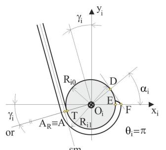
Sm Figure 5 – Determining the angle  $\alpha_i$
