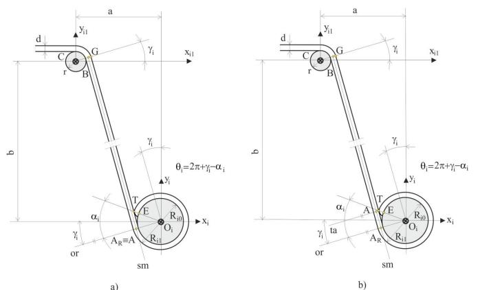
Figure 6 – Position of the system for:  $\theta_i = 2\pi + \gamma_i - \alpha_i$ , a) the last moment of *con* area, b) the first moment of the *jumpvar* area.
