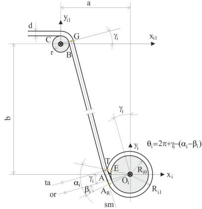
Figure 7 – Position of the system for:  $\theta_i = 2\pi + \gamma_i \cdot (\alpha_i \cdot \beta_i)$ .
