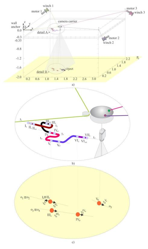
Figure 1. The RSCPR system's camera tracking and monitoring a chaotically moving object: a) 3D view, b) detail A: detailed view of the camera trajectory, c) detail B: detailed view of object's positions.
