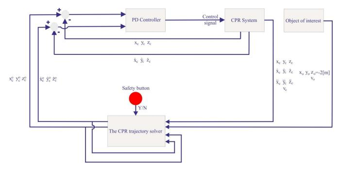
Figure 3. Block diagram of the trajectory choosing process.
