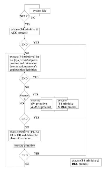
Figure 4. Flow chart of the CPR Trajectory Solver.
