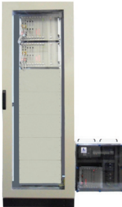
Figure 2 - Overview (frontal) of the turbine regulation (left) and hardware simulator (right)
