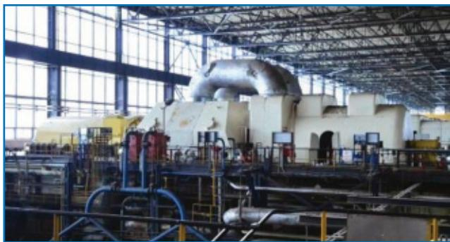
*Slika 1 - Parna turbina bloka TENT A2, 210 MW*
